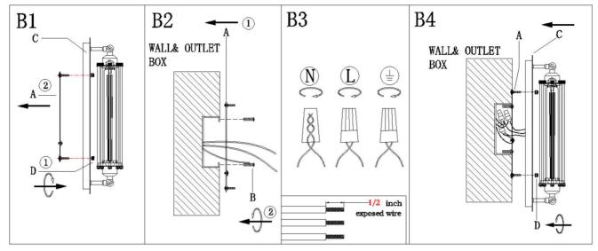
Step B1: Unscrew ball nuts (D) from back plate (C) then gently remove mounting plate (A).
