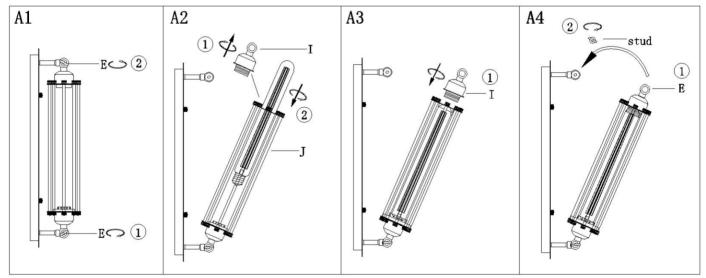
Step A1: Slightly loosen the stud in lower joint (E) and allow it to rotate a little bit.
