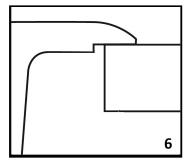
Place a bead of a good quality silicone on the underside rim of the sink. Locate the sink correctly in the cutout in the countertop. Place some weight (about 10lbs) in the bowl to provide pressure while the silicone cures. Wipe up excess silicone with a damp rag before it dries.
