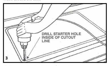
Drill a starter hole just inside of the cut line.
