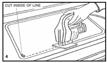
Use a jigsaw to make the cutout. If you are using a countertop material other than laminate, you will need to use the appropriate router and hard surface template to accomplish the cutout.
