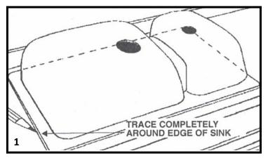
Use the sink as your template. Place sink upside down in the position where sink is to be installed. Pay attention to the backsplash, faucet placement and vanity cabinet constraints. Trace around the sink.
