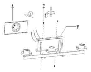
Step 2:Carefully pass outlet box wires through mounting plate (A)
