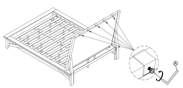
To attach the upholstered pad, remove the four bolts with washers using the allen wrench provided, then place tab grommet over the hole and replace bolt and washer.
