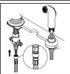
(4) Guide the side spray hose through the side spray holder. Insert the side spray hose quick connect adapter into faucet outlet end, push until a "click' is heard. Pull side spray hose downward to test engagement.
