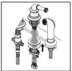
(5) Place cold and hot side valves in position on the sink, ensure handles operate in correct direction. From underneath of the sink handtighten locknut to the faucet. Position faucet to desired location from top. Tighten screws on locknut with the help of Phillips head screwdriver to secure faucet.
