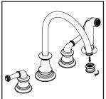
(6) Important: After installation is complete, remove the aerator. Turn on the water and allow both hot and cold water to run for at least one minute each. While water is running, check for leaks. Turn off the water and replace the aerator when finished.
