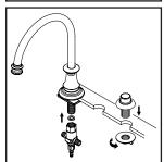
(3) Thread Cross connector to the spout shank. Ensure there is a washer in the Cross connector. Do not overtighten. For faucet with side spray, Place side spray holder on mounting hole. Tighten locknut from underneath the sink to secure side spray holder.
