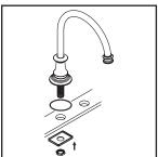
(2) Make sure O-ring is under escutcheon. Insert spout with spout escutcheon into mounting hole. Slide mounting plate through spout shank and tighten with locknut from underneath the sink.
