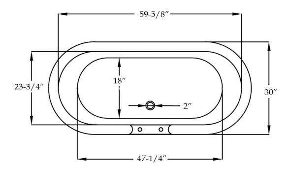
Weight (empty): 341 lbs Weight (filled): 869 lbs Capacity: 58 gal Water depth: 15"
