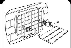
**3. MOUNTING** (Masonry, brick, block wall) 16" on center (use template provided). Install 6 plastic wall plugs provided. A 0.4" diameter masonry drill should be used for this application.
