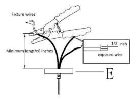
6 » Carefully pass supply wires through mounting plate assembly (A).
