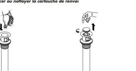
4. Remove cartridge (2) from drain:
