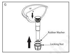
G. Remove rubber washer and locking nut from the drain assembly and slide the drain into the sink. Install the rubber washer first and tighten the locking nut to install the drain. Connect the drain to the P trap and waste pipe.
