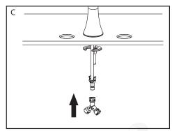
C. Insert the Tee connector to the center spout inlet hose until it clicks in place. Make sure the hose is fully inserted. There will be an audible click when the connector is connected properly.
