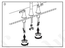
D. Slide hot and cold water handle through the 2 side mounting holes. Handles should point outward in off position. Secure the handles with the mounting nut.
