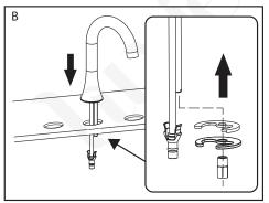
B. Place spout through the center mounting hole on the surface. Secure spout with C shaped washer, C shaped metal washer and locking nut.
