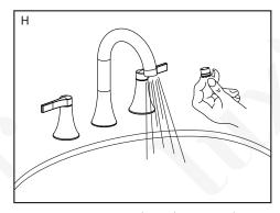
H. Turn on water supply and remove the aerator with a small coin or a flat head screwdriver and let the water run for about 1 minute to clear any debris in the plumbing system. Check for leaks at all connections. Reinstall the aerator to complete the installation.
