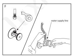
F. Apply Teflon (PTFE) tape on the shut off valves. Thread the tape in counter-clockwise direction. Use a wrench to tighten the hoses. Please do not overtighten the connections.
