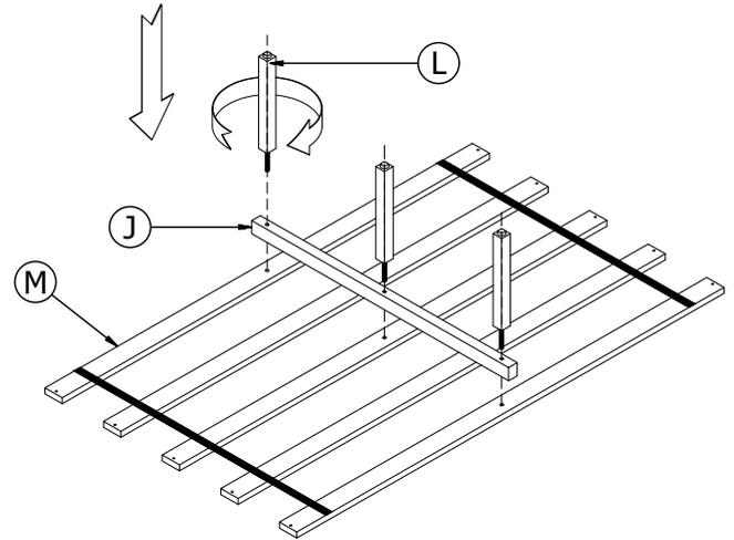
Step 6. Set Slat roll(M), link pre-wire up. Next, place the Long center support slats(K), align the drill holes.
