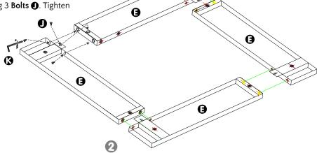
Assemble the fire pit base by attaching each Side Panel (2) to 2
