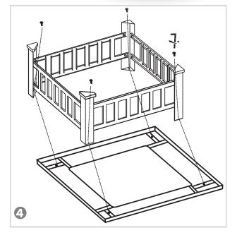
Turn the assembled frame upright and place the Fire Bowl into the frame, then place the Wood Grate in the Fire Bowl.
