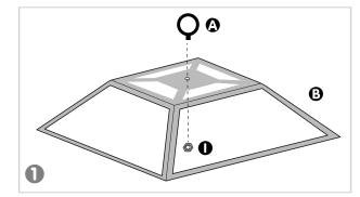
Assemble the tabletop by arranging the **Tabletop Panels (3** upsidedown as shown, then securing each joint using 3 **Bolts (9**). Tighten each **Bolt** using the **Hex Wrench (6**).
