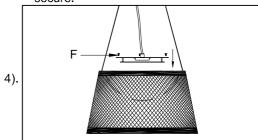
Step.4: Secure lamp Shade (E) to Body (D) using screws (F) provided.
