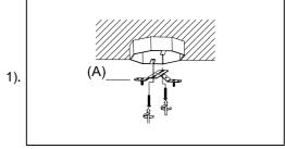
Step.1: Remove mounting bracket(A) from fixture and install to electrical box.
