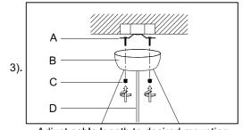
Adjust cable length to desired mounting Step.3: height, and tighten strain relief screws to secure. Install body (D) to bracket (A) and tighten finials (C) on the canopy (B) to secure.
