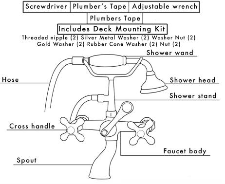
It is always advised to place plumber's tape on all threaded areas. 1. Assuming your water lines are prepared. Locate a threaded nipple, one silver metal washer, and a washer nut from the deck mounting kit. Slide the metal washer down the nipple and thread the washer nut onto the straight end of the nipple.
