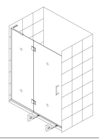
**25.** With the door open, apply a good quality mildew-resistant/waterproof silicone along the connection of both U-Channels to the wall and threshold on the inside of the shower.
