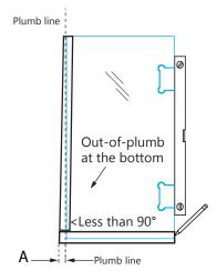
\*\*If the wall is out-of-plumb at the <u>bottom</u>, measure that dimension as (A) and add it to the length of the U-channel ( +1/4" max):
