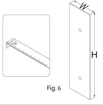
NOTE: The top of the Enclosure glass must be level with the Glass door. By using a level across the top of both the In-line Stationary panel glass (11) and door, height differences can be measured. The Adjustment spacers (28) are provided for the Return panel glass (26) only to compensate for such differences by inserting them into the U-Channel 2 (bottom profile) (29). Please use the correct spacer size that is needed for your situation.
