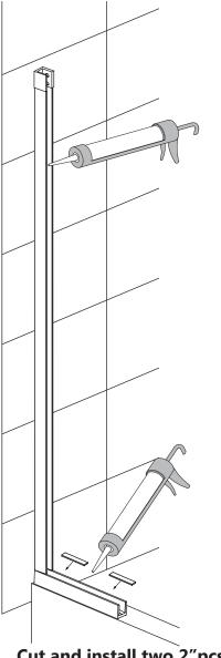
Cut and install two 2"pcs of the 0.5 mm shims (#34) into the bottom U-channel to protect the corners of the glass
