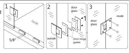
Set the **Door Glass (#01)** with the **5/8**" spacers attached onto the threshold, inline with the **Hinge Panel Glass (#32)**. Level up the **Door Glass (#01)** with the **Hinge Panel Glass (#32)** and fasten the hinges onto the **Door Glass (#01)** using one 2mm hinge gasket per side. Make sure the top edges of the **Door Glass (#01)** and **Hinge Panel Glass (#32)** are aligned and that there is an even reveal between the door and panel glass.
