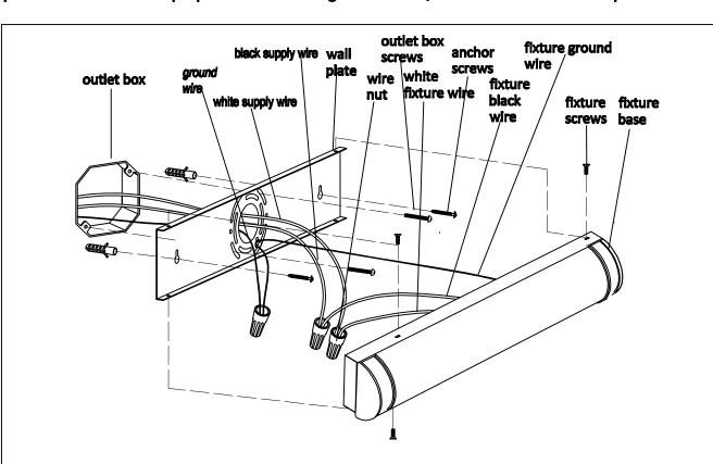
1: Place the mounting wall plate over the outlet box, align the mounting slots of the wall plate with holes of the outlet box as shown. Use a level to ensure the wall plate is straight.
