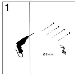
For drywall installation, mark the hole locations and drill  $\Phi$  6mm holes for the drywall anchors. Install a junction box behind the mirror for power connections.
