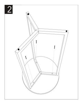
Step 2 Screwing the leg (A) in to the table top (B)
