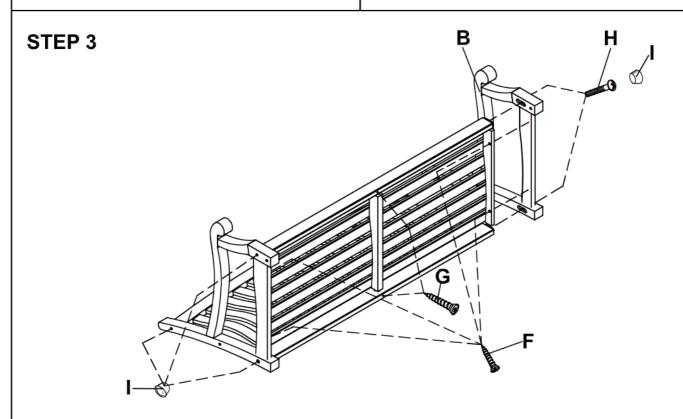
Attach the left armrest (B) to the assembly from step 2, secure using 1 1/2" bolts (H), 1" screws (F) and 1 1/2" screws (G) from underneath, position as shown, tighten using screwdriver. Tap in wooden caps (I) to cover bolt heads using rubber mallet.
