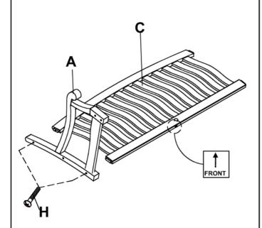
Install on level ground. Attach the right armrest (A) to the back rest (C), secure using 1 1/2" bolt (H).
