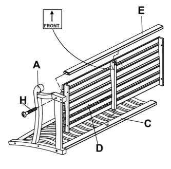
Attach the apron (E) onto the seat (D). And then attach the seat (D) onto the back rest (C) and to right armrest (A) secure using 1 1/2" bolts (H), position as shown.
