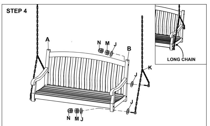
Secure the hanger bolts with chain (K) into predrilled holes of left armrest (B) using washers (J), nuts (M) and head nut (N), as shown. (The hanger bolt with long chain must be installed in front, short chain must be installed at the back).
