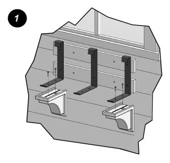
Secure each decorative bracket to the bottom of the wall mount brackets using two 1 inch screws. The decorative brackets are sold in pairs so we recommend installing them on the outside brackets as shown above.
