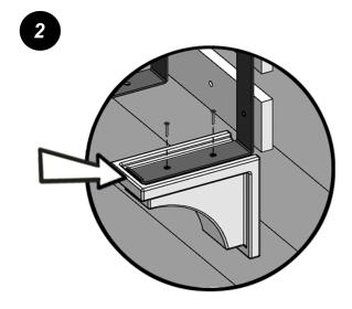
The front lip of the wall mount bracket should sit flush against the inside face of the decorative bracket (indicated by the arrow). The molded brackets are only decorative so there is no need to over tighten the screws.
