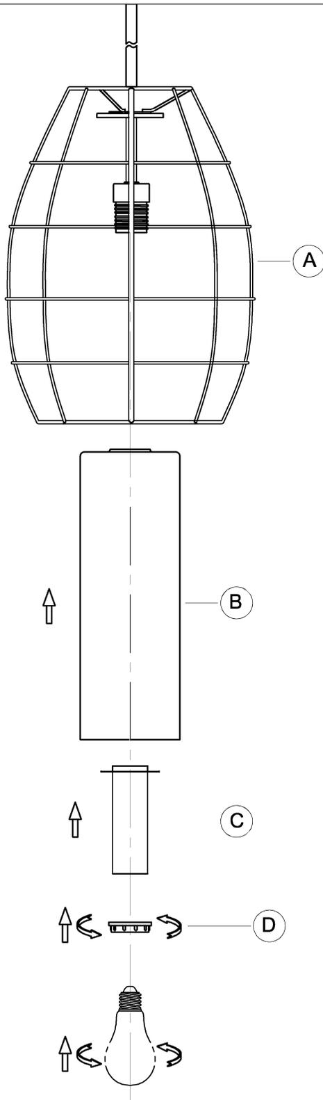
6. Attach glass shade (B) to fixture (A) using socket spacer (C) and socket ring (D) to secure tightly.
