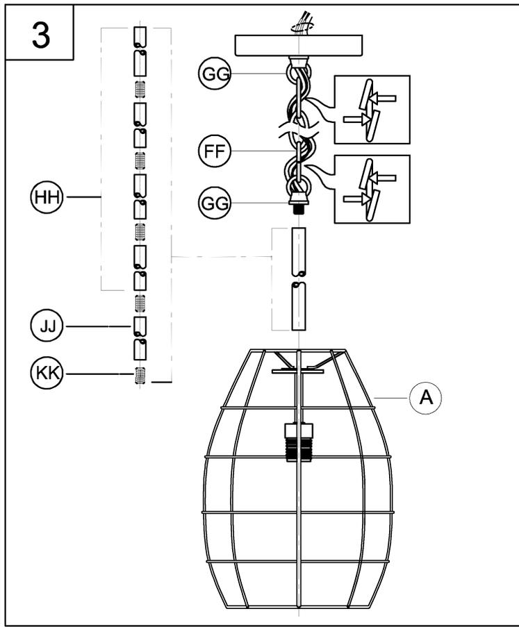
3. Pass the wires through the nipple (KK)/one pipe (JJ)/four pipe (HH) and Chain loop (GG) to achieve overall desired length. Next attach pipe onto fixture (A) use nipple (KK) to secure tightly. Weave electric cord and ground wire through chain loop (GG) and chain (FF). Open two links of chain and attach both ends to chain loops (GG). Close the chain links.
