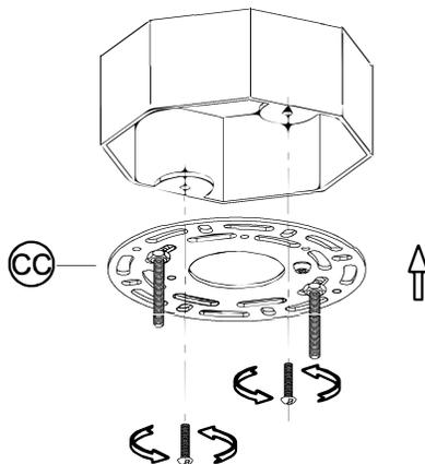
2. Attach assembled parts from step 1 onto outlet box using the mounting screws supplied with the outlet box (not included).
