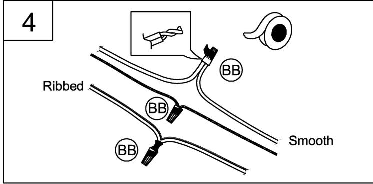
4. Strip 3/8" of insulation from the electrical wire ends. Using wire nuts (BB), connect RIBBED fixture wire to the WHITE supply wire from the junction box; connect the SMOOTH fixture wire to the BLACK supply wire. Connect the fixture ground wire and supply ground wire using a wire nut or by fastening to the ground screw on the round mounting plate. Push all wire connections into the outlet box.
