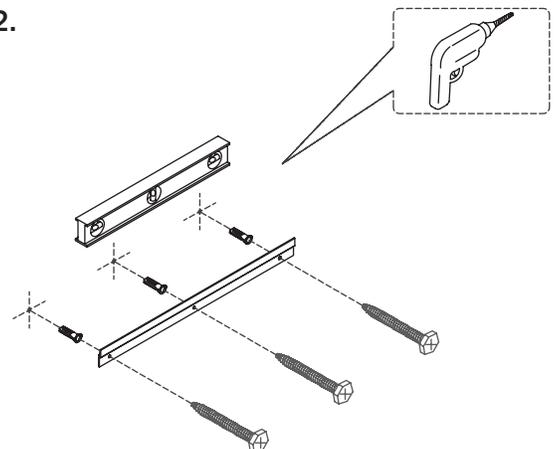
**Step 3:** Secure the anchors in the wall, and then fasten the screws provided into the anchor to secure the wall cleat.
