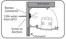
Secure APS – TR Series to wall with screws into each stud or use anchors provided. Strip wires and connect Black wire from romex to Gold terminal and White wire from romex to Silver terminal. Ground all Green wires to PEM studs inside of back frame. When connecting two APS – TR Series, run Romex from piece A to piece B. Ground each section to the next.
