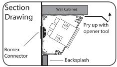
Turn power off at panel. Carefully pry open each piece with tool (provided). Insert Romex connector into hole. Pull wires into APS-TR Series.
