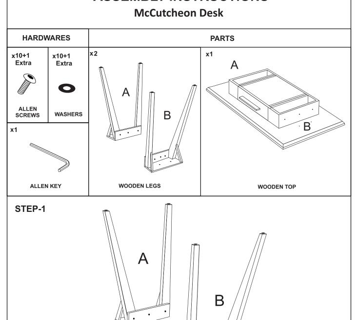
Place top face down on a protective surface. Align 2 legs (A& B) as indicated.
