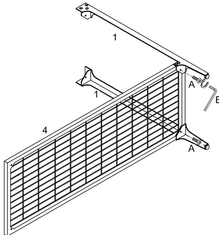
Attach legs (1) to frame (4) using bolts (A) as shown in the diagram.
