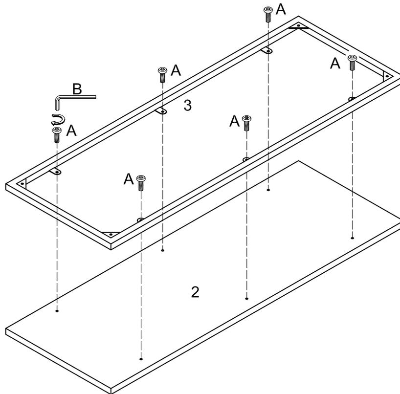
Secure wood panel (2) to frame (3) using bolts (A) as shown.
