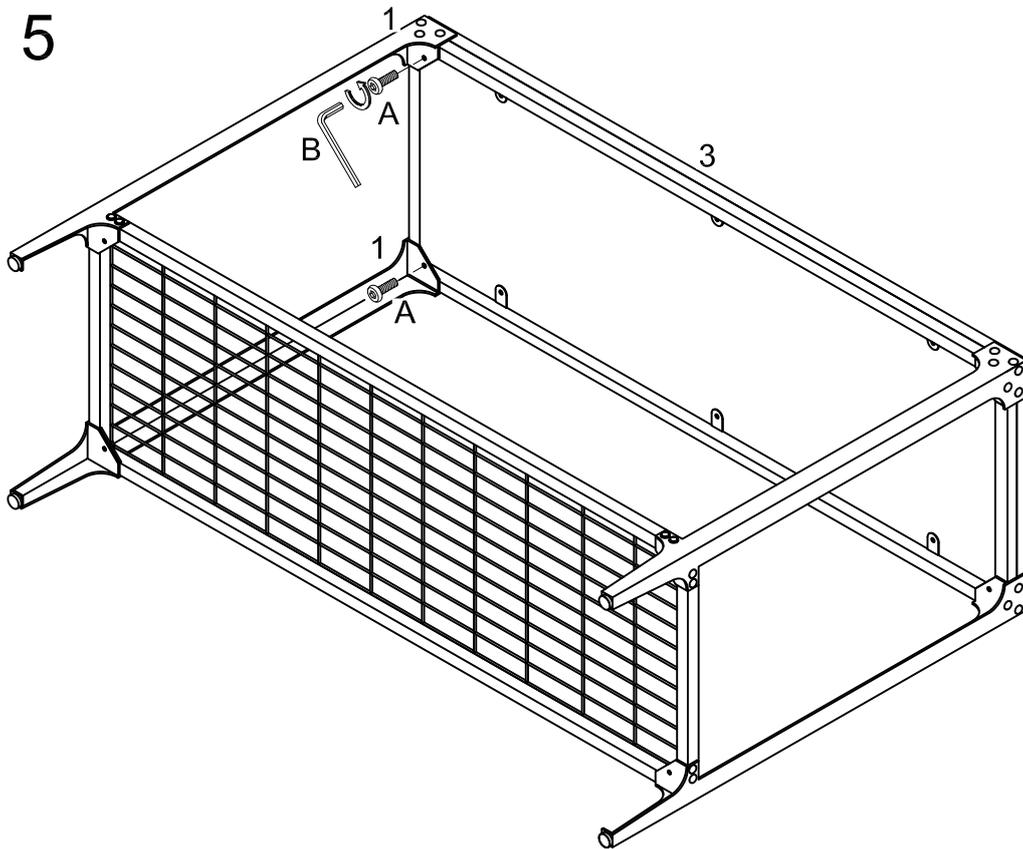
Attach frame (3) to legs (1) using bolts (A) as shown.
