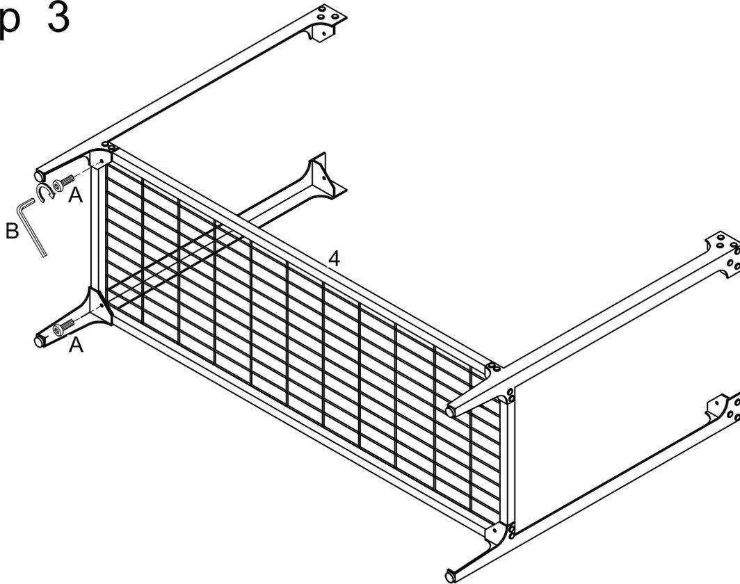
Attach legs (1) to frame (4) using bolts (A) as shown in the diagram.
