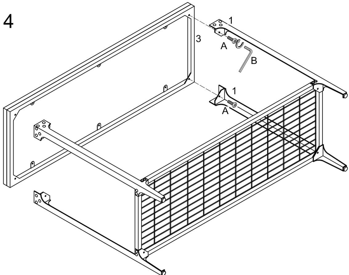
Attach frame (3) to legs (1) using bolts (A) as shown.
