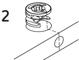
You should insert these cams with the little arrow pointing towards the drilling on the panel's edge (shown on the left).
