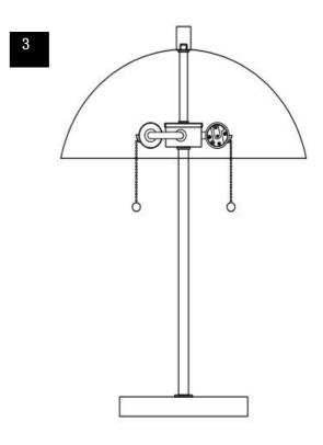
Step 1 Pull power cord to connect the Center Tube (B) to the Base (A) Insert the Pole (D) into the Socket Assembly (C). Screw the Center Tube (B) onto the Lamp base (A) Screw the Socket Assembly (C) onto the Center Tube (B). Be careful not to twist the power cord and tighten securely
