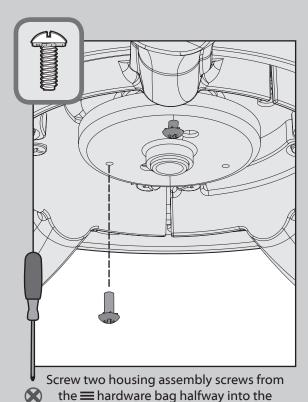
motor housing. It does not matter which
