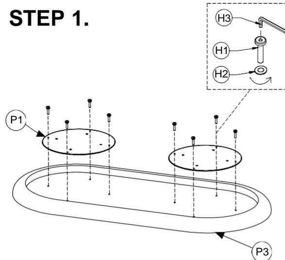
\*Screw the bolts out to take frame out (P1) of top (P3)
