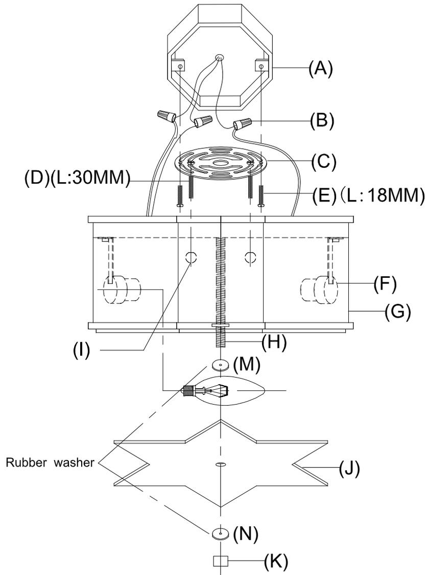
1. Connect the hot wire from the fixture (BLACK) to the hot wire from ceiling outlet box (A) (usually BLACK). Fasten them together with a plastic wire connector (B) provided and wrap connection with electrical tape.
