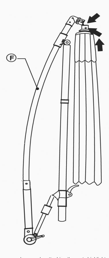
Assemble the parasol canopy by attaching the parts highlighted above. Make sure the sprung nipples lock into place securely. You may need to turn the crank handle to tighten the cord so it does not become trapped.
