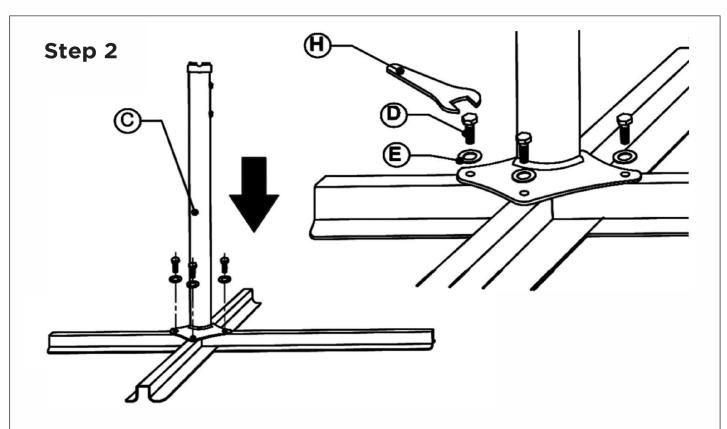
Attach the base stand (C) to the feet using four bolts (D) and four washers (E). Tighten the
