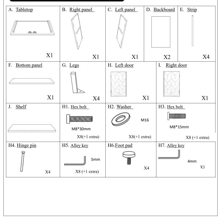
Step 1: Put the Tabletop (A) on a soft surface to protect the finish. Attach the Left & Right panel (B&C) with Hex bolts (H1) and Washers (H2) using Allen key (H5). The Door hinge on the Left & Right panel (B&C) should be aligned on the same side as the Magnet on Tabletop (A). Ensure the groove on Left & Right panel (B&C) aglined with the groove on Tabletop (A).Leave hardware loose in this step.
