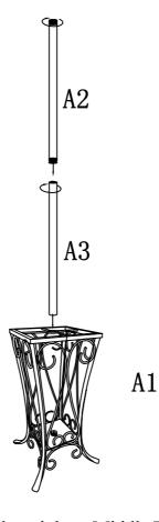
Tighten Lower Rod A3 to Base A1, then tighten Middle Rod A2 to Lower Rod A3 as shown above.
