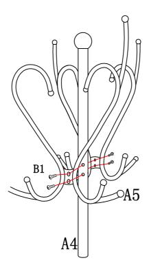
Attach Hooks A5 to Upper Rod A4 using Bolts B1.
