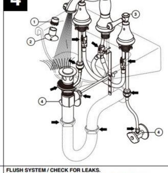
Remove aerator (1) using supplied wrench (2) and turn faucet handles (3) all the way on. Turn on hot and cold water supplies (4) and flush water lines for one minute. Important: This flushes away any debris that could cause damage to internal parts. Check all connections at arrows for leaks. Re-tighten if necessary,
