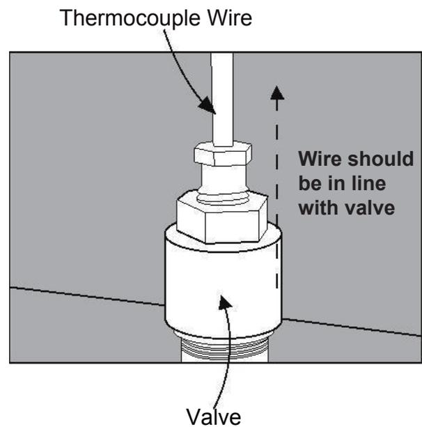
4. Make sure that the thermocouple wire is correctly positioned. The thermocouple wire should be in line with the valve.
