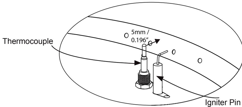
3. Make sure that the igniter pin and thermocouple are correctly positioned.
