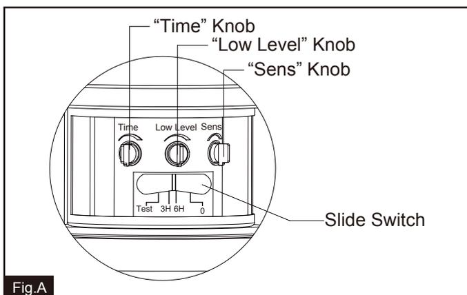
Step 1: Rotate the sensor lens from left side to right side to show the adjustable knobs and slide switch. (See Fig.3)
