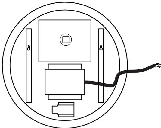
**Electric wiring:** Be sure to provide enough wire to make the proper and safe connection to the Field/Power.
