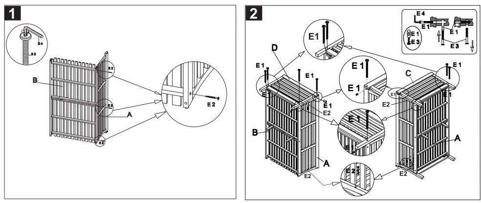
Step 1: attach the seat (B) to the back (A) by using the Allen Screw (E2) and tighten with the Allen Key (E4).
