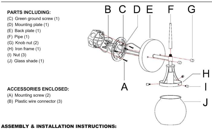
1. Carefully remove the fixture from the carton and check that all parts and accessories are included as shown in the above illustration.
