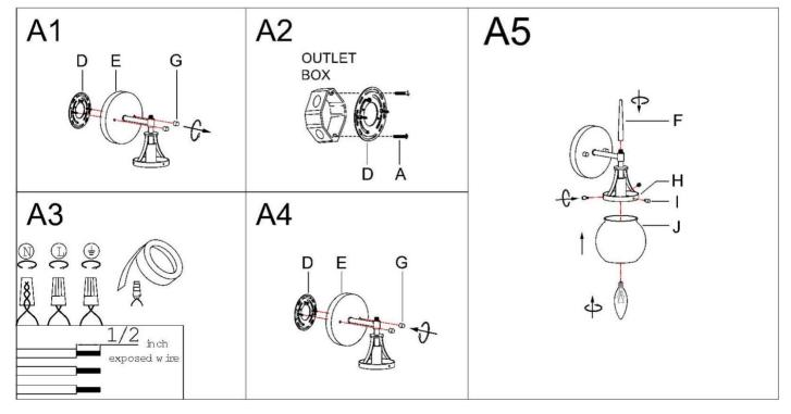
Step A1 » Unscrew knob nuts (G) from back plate (E), then set them aside for later installation.
