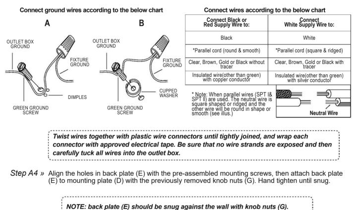
If not, remove back plate (E), adjust the threaded length of pre-assembled mounting screws on mounting plate (D):
