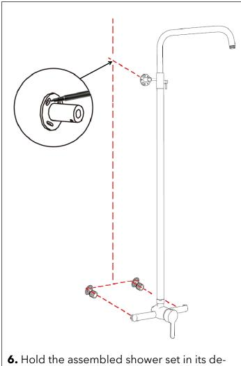
**6.** Hold the assembled shower set in its desired position and mark the location of the mounting bracket.
