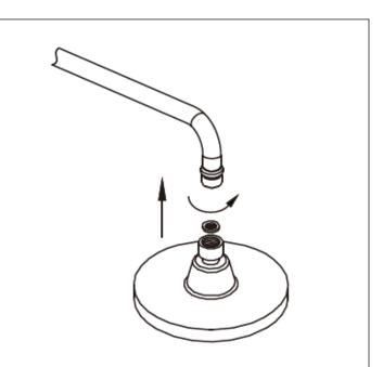
**12.** Install the rain shower head. Make sure to use a sealing washer.
