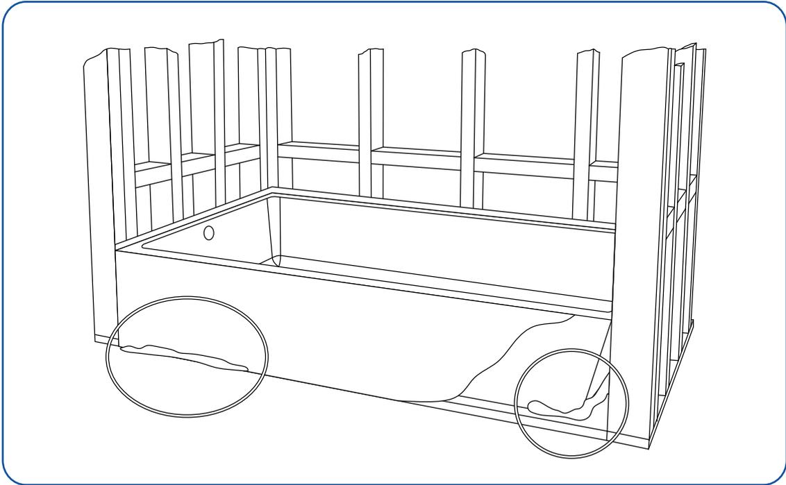
19. Apply pressure to the tub's center until the mortar solidifies.
