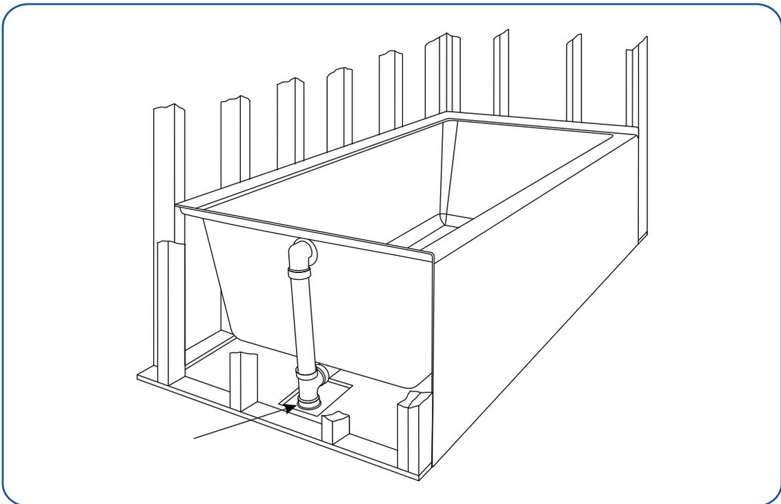
24. The tiling flange is not designed to support the bathtub's weight; it **MUST** be fastened to the studs. It is advised to pre-drill the flange to prevent the acrylic from cracking.
