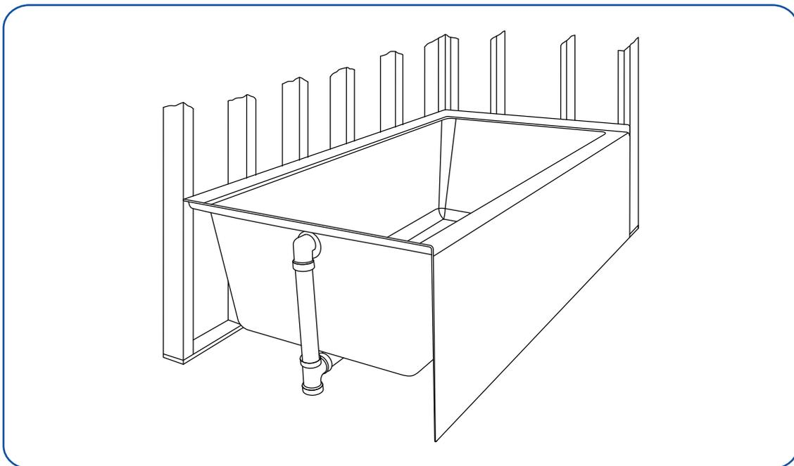
Two common methods for securing the bathtub are a mortar bed or construction adhesive. Alternative methods are also available, depending on the specific installation site. Please consult with a certified plumber/installer.
