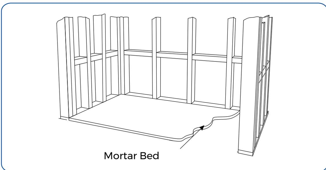
14. The bathtub must be fully supported at its base and anchored to the floor using either a mortar bed or construction adhesive.
