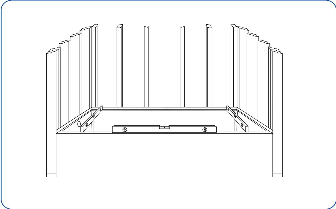
7. Mark the drain's position and the overall height of the bathtub on each stud located above the back horizontal integrated tiling flange.
