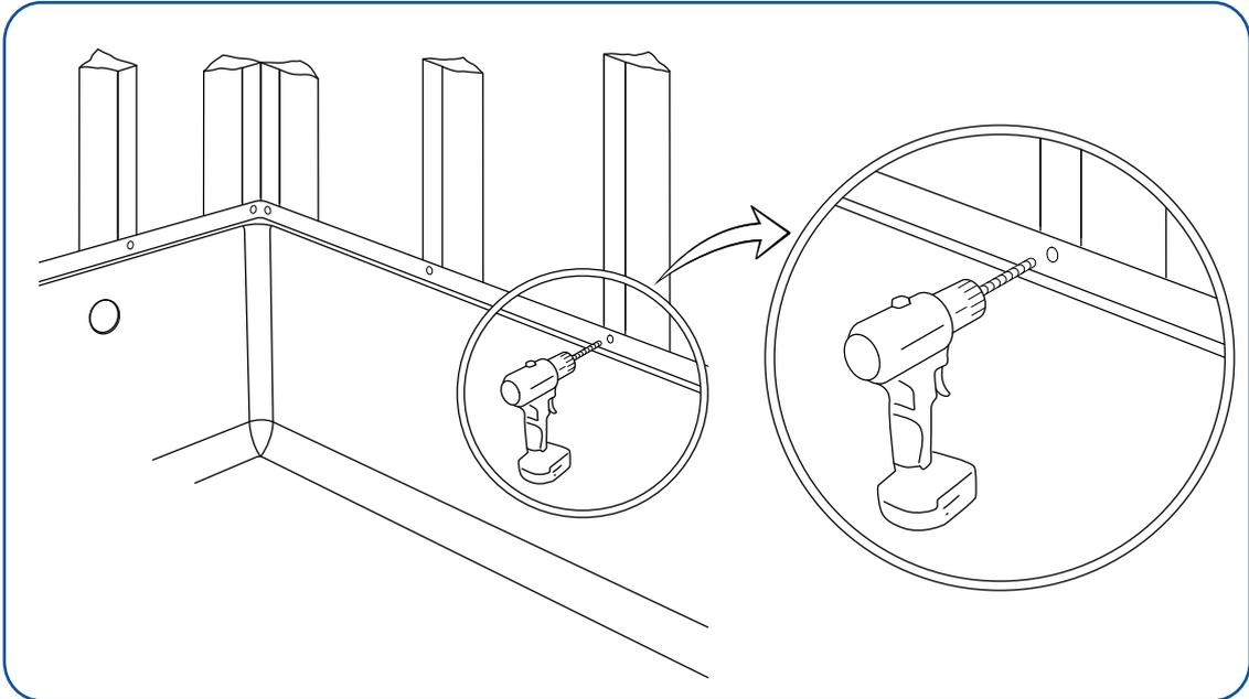
26. After drilling, apply silicone to the tiling flange holes to guarantee a watertight seal.
