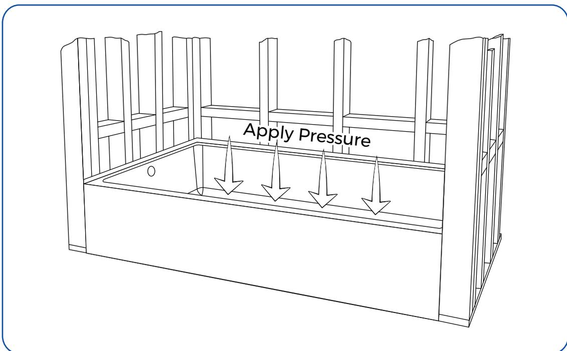
20. Ensure the bath is level across the top and is plumb along the drain side. Adjust if necessary; if unlevel, use shims beneath the blocks.
