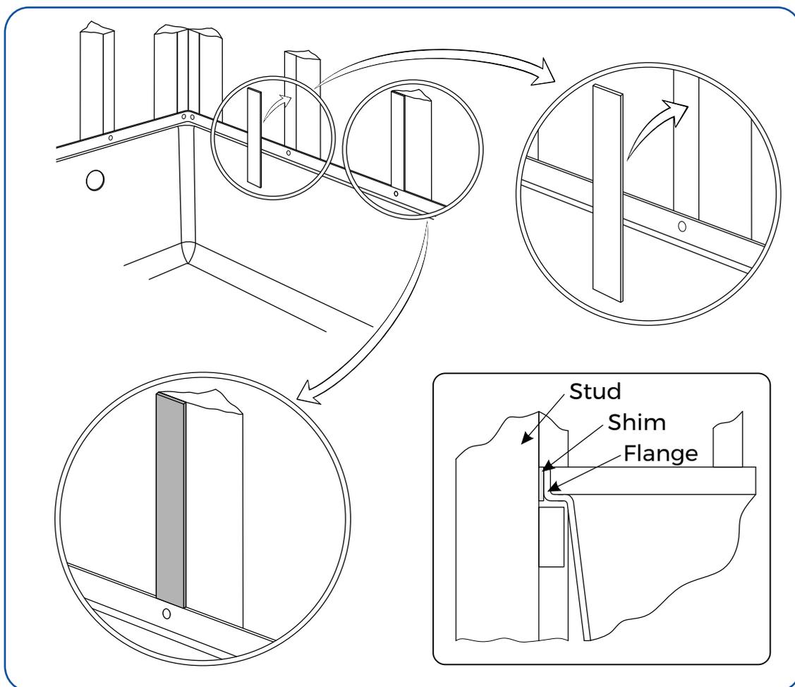
28. Ensure gaps between flanges and studs are under 1/8" after shim placement.
