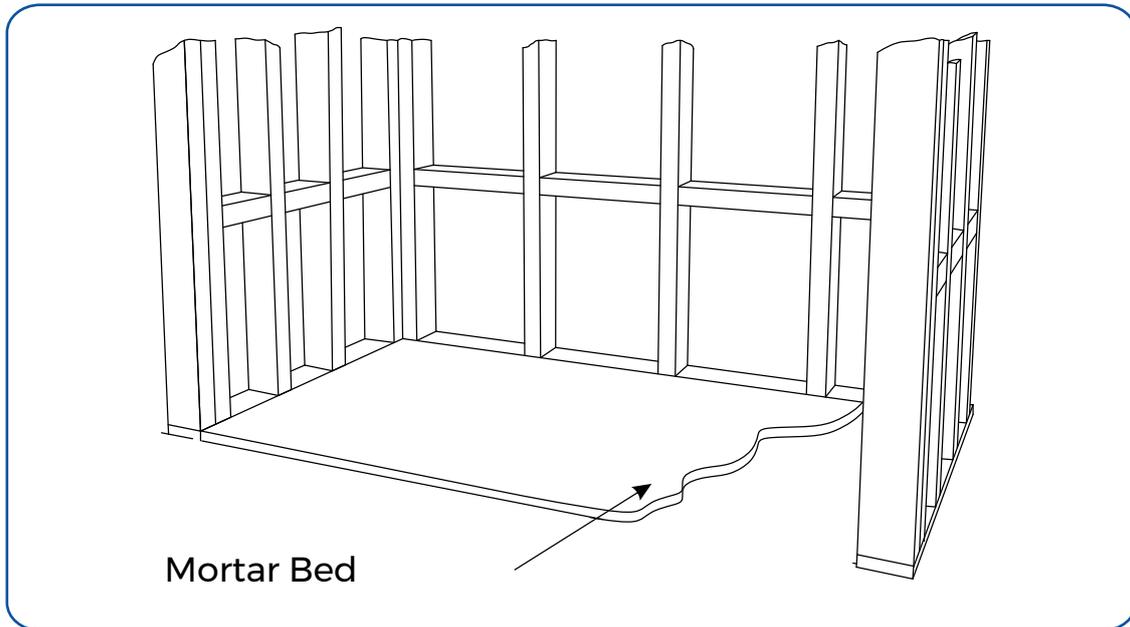
16. Distribute the mortar across the floor, avoiding the spots where the leveling feet will be positioned.
