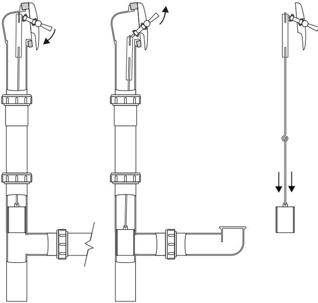
1. Insert the linkage assembly into the overflow, ensuring the trip lever is in the open position (Facing down).
