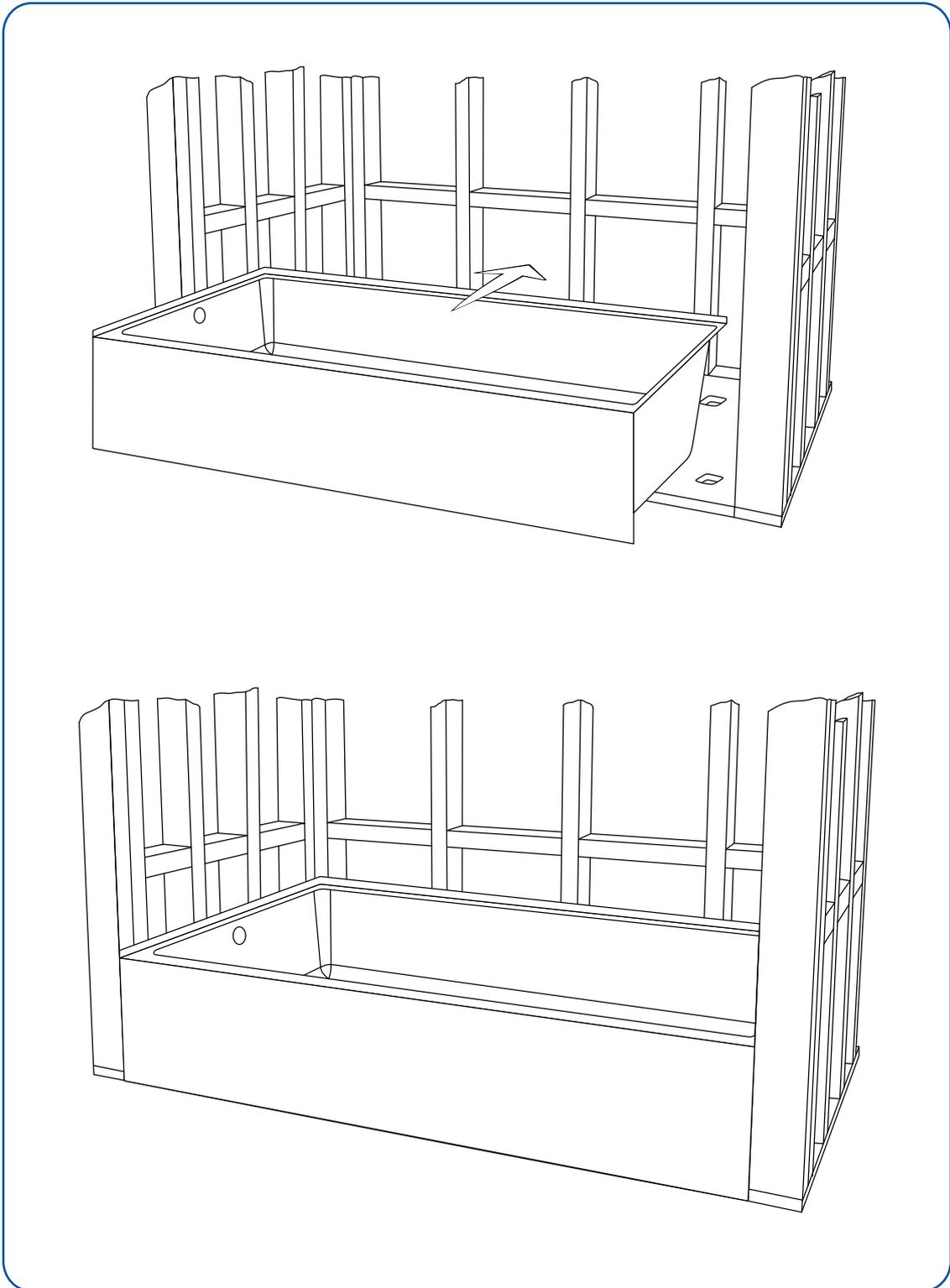
18. Let the bathtub settle into place, being vigilant of any excess mortar accumulating on its sides and ends.
