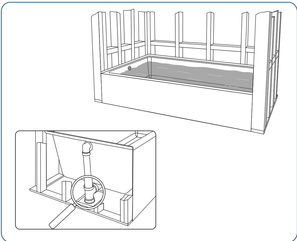
31. Mount water-resistant drywall on the framing and seal seams with 100% silicone sealant. Make sure to position the finished wallboard over the tiling flange, leaving a  $\frac{1}{4}$ " (6mm) opening, which creates a groove for the silicone sealant.
