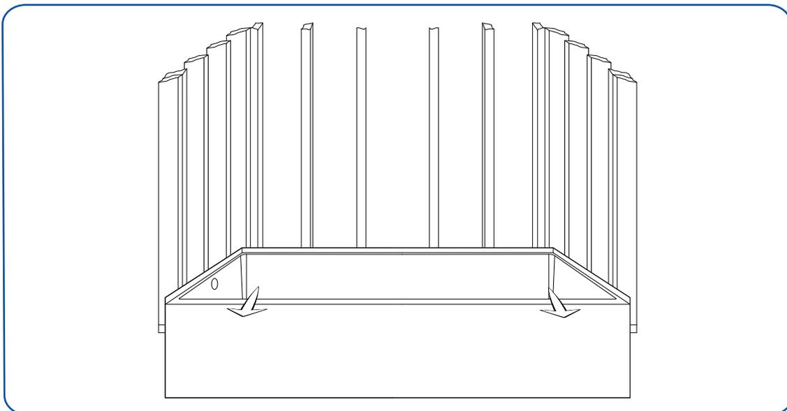
10. Starting from the previously marked overall height, measure and make a mark just below, indicating the appropriate height for the leveling stringer. This stringer will provide additional support beneath the tiling flange when securely attached to the stud wall.
