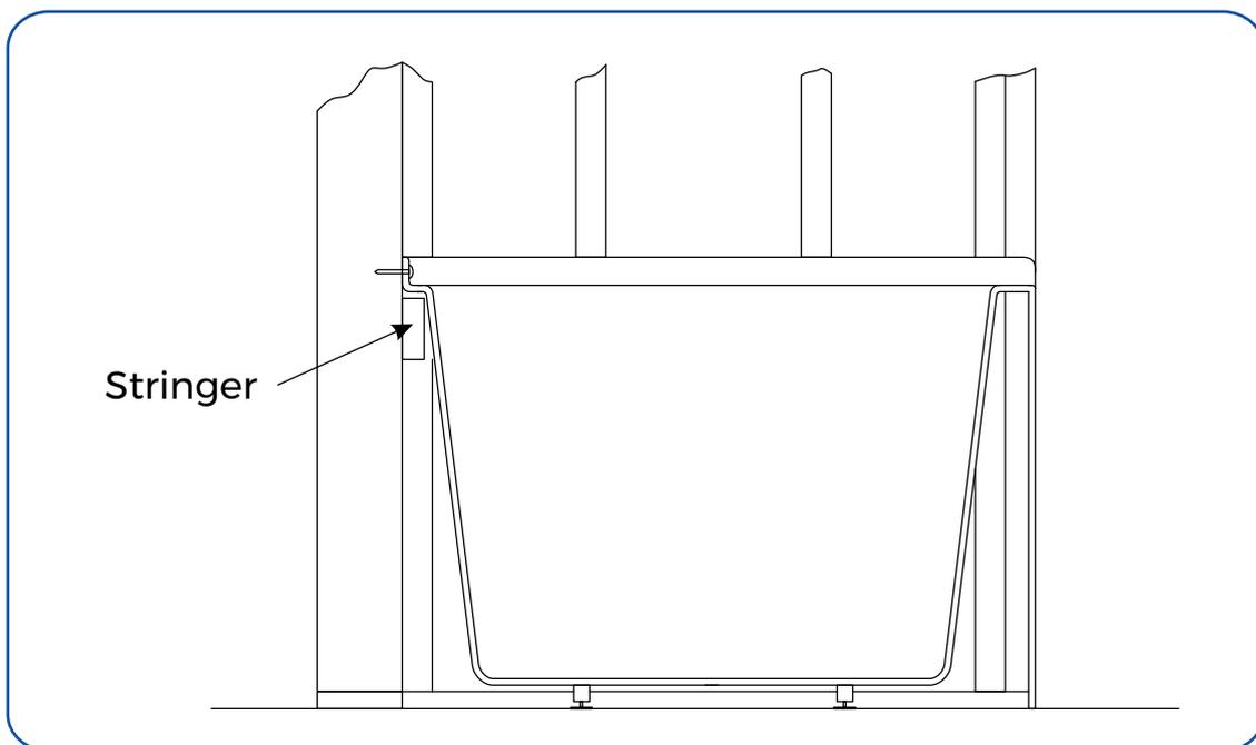
11. Dry fit the bathtub in the plumb socket and check again for level.
