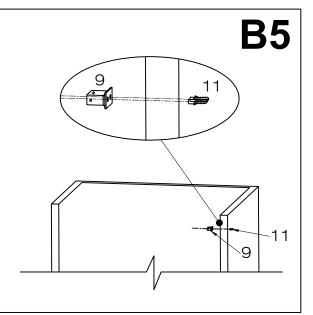
Screw the wall connector (#9) into the white plastic anchors (#11) with the 1 5/8" hex screws (#10).
