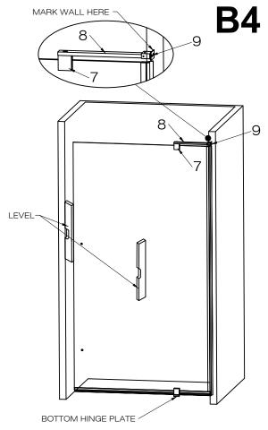
5. Remove the wall connector (#9) from the structural arm (#8) and place against the wall where you've marked. Mark the holes for the wall connector and remove. Drill holes into the wall where marked. Place white plastic anchors (#11) inside the holes.
