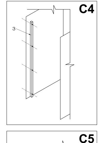
5. Remove the vertical rail, pre-drill and sink plastic anchors (#1) into the wall. <u>Not</u> necessary if installing into studs. Studs are the preferred means of installation, anchors can pull out of the wall causing property damage and bodily harm.
