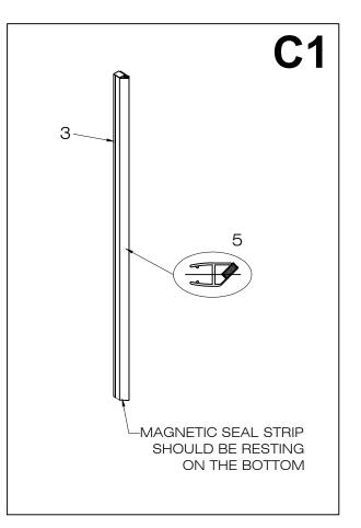
2. Attach the door magnetic seal strips (#5) to each other and then close the door, making sure the door is on a level plain, keeping the walls and opening at a perfect 90° angle.
