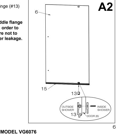
Place the bottom part of the bottom hinge (#13) on the floor \*10 1/4" from the wall. Mark the holes on the floor. Remove the piece and drill holes into the floor where marked. Place green plastic anchors (#1) inside the holes.
