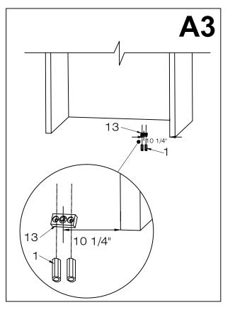
4. Screw the bottom plate of the bottom hinge (#13) into the green plastic anchors (#1) with the 3/4" phillips screws (#14). <u>I</u> It is imperative that you install the piece properly depending on which direction the door opening is. Please refer to page 5 for the proper configuration.
