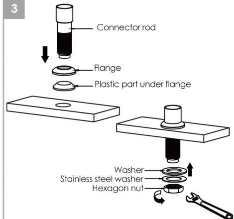
Introduce connector rod into hole, ensure flange and plastic rubber are above the countertop. Secure connector rod with hexagon nut, firmly with a wrench.
