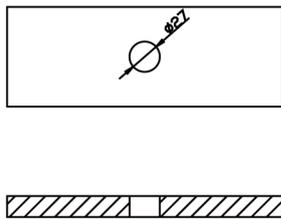
Recommend hole size 27mm to 35mm hole diameter.
