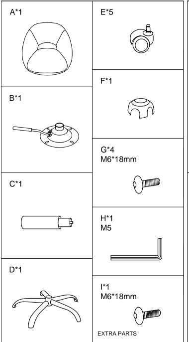
1 Insert casters E to bottom of the spider base D. Attach the metal cover F on top of the spider base D then insert the gas lift C to the center hole of the base D.
