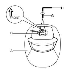
3 Attach the whole seat to base assembly, make sure top of gas lift align with center hole of mechanism B under seat.
