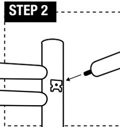
**STEP 2:** Use the short mounting screw (d) to fix the mounting tube (a) to the threaded metal pad on the vertical bar on the back of the towel warmer.
