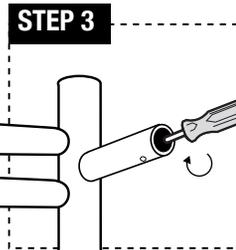
**STEP 3:** Screw down the short mounting screw (d) with a screwdriver. Note that the set screw of the tube (a) should point towards the floor when the towel warmer is wall mounted. Fix the remaining two mounting tubes (a) to the vertical bars with threaded metal pads by repeating Step 1-3.
