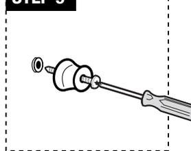
**STEP 9:** Insert long screw (i) through mounting bracket (g), then screw into plastic drywall anchor (f).
