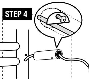
**STEP 4:** Guide the electrical cord through the electrical connection mounting tube (b) and use the long mounting screw (e) to tighten the electrical connection mounting tube to the vertical bar.
