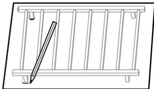
Place towel warmer on the box (or a large sheet of paper) and lay on a flat surface with mounting tubes facing downwards. Mark the location of the following:
