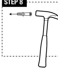
**STEP 8:** Use a hammer to knock plastic drywall anchor (f) into wall completely.
