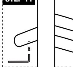
**STEP 11:** As shown in the picture, install the set screws (c) into the hole of all the tubes (a and b) using the allen wrench; fix the tube (a) onto the mounting bracket (g and h).
