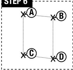
**STEP 6:** Mark A, B, C, and D according to the data from Step 5; It is suggested that this product be installed at least 23.5 inches (59.69 cm) above floor level. (WARNING: The electrical connection should avoid all water). This mounting location must comply with all local building and electrical codes.
