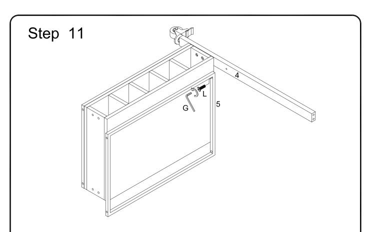
Attach part (5) to part (4) using bolt (L) with hex key (G).
