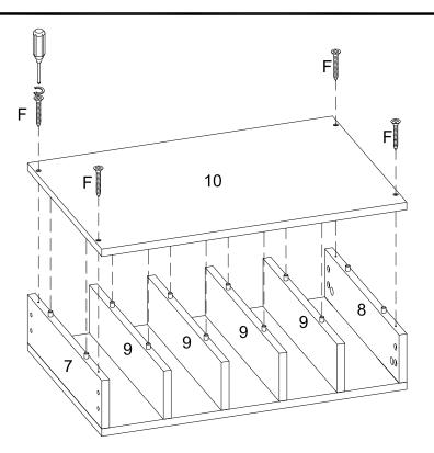
Insert part (10) into part (7,8,9), then secure part (10) to part (7,8) using screw (F) with screwdriver.
