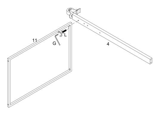
Attach part (11) to part (4) using bolt (L) with hex key (G).
