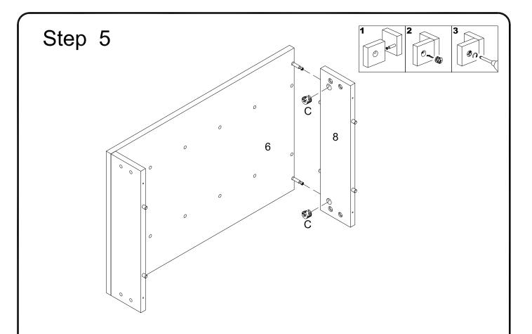
Attach part (6) to part (8), then insert and secure cam lock (C) to part (8) to lock it.
