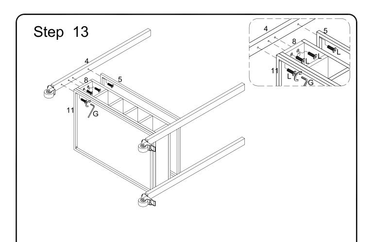
Attach part (5,8,11) to part (4) using bolt (L) with hex key (G).
