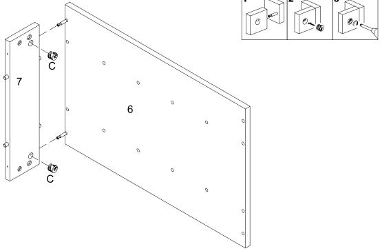
Attach part (6) to part (7), then insert and secure cam lock (C) to part (7) to lock it.
