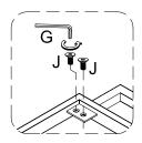
Attach part (2) to part (4) using bolt (J) with hex key (G).
