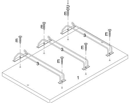
Attach part (3) to part (1) using screw (E) with screwdriver.
