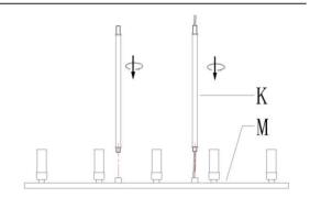
4. Thread stems (K) through upper ring (J), then screw the tubes (I) to the top of stem (K) until tight.
