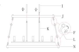
5. According your desired hanging length to choose and use the tubes (I). Pass wires through the chosen tubes (I) ,loop (G) and canopy (E). Screw the tubes (I) onto the previously installed tube until tight . then attach a quick link (F) to connect the canopy (E) and tube (I) together.
