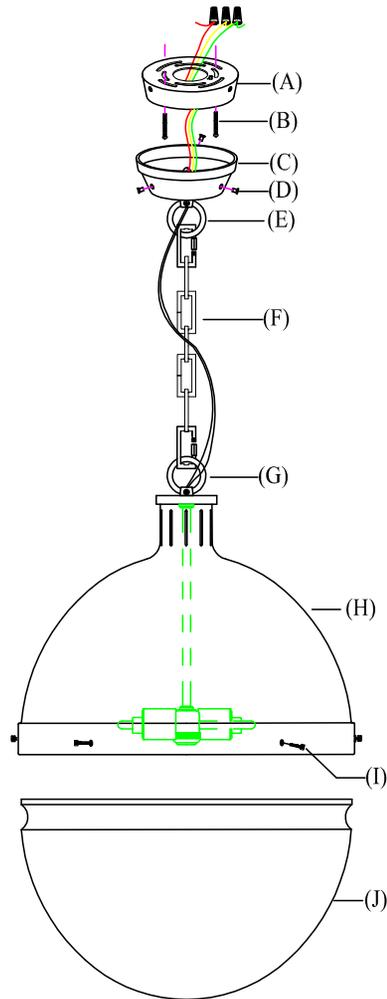
1. Attach chain (F) to top loop (G) by opening and re-closing end link of chain. Feed wire through chain (F) and canopy (C). Attach chain with fixture to chain mounting loop (E) at desired height.
