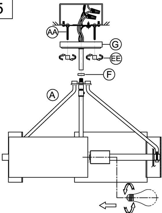
5. Attach seat ring (F) onto fixture (A), thread fixture (A) onto canopy to secure tightly.
