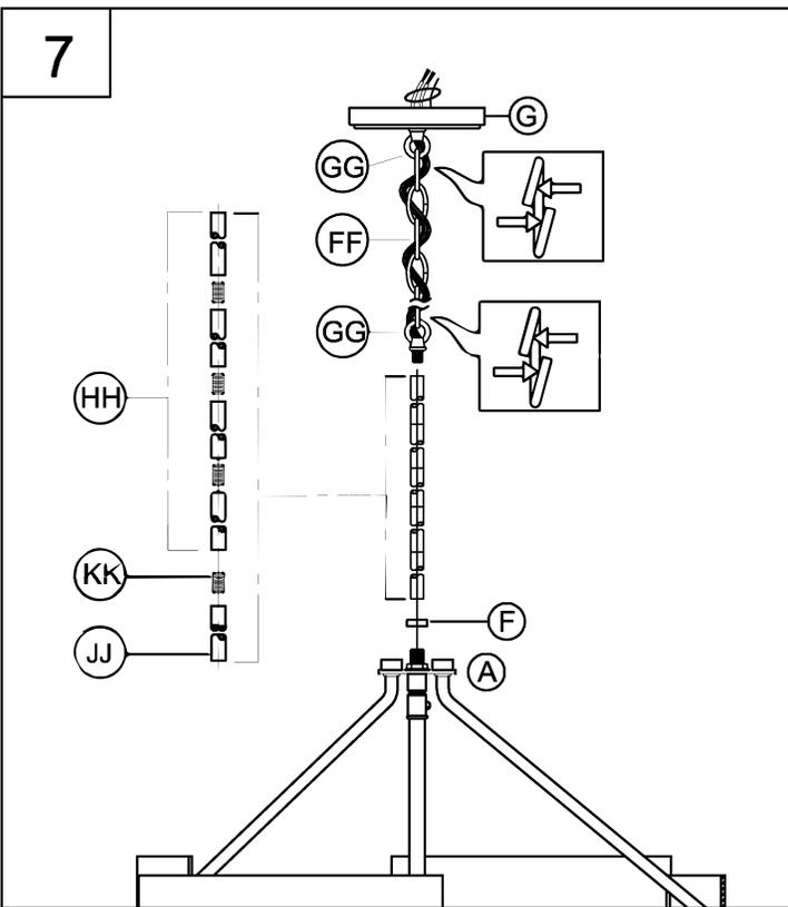
7. Pass the wires through the seat ring (F) / nipple (KK)/one pipe (JJ)/four pipe (HH) to achieve overall desired length. Next attach seat ring (F) / pipe onto fixture (A) , secure tightly. Weave electric cord and ground wire through chain (FF) and chain loop (GG). Open two links of chain and attach both ends to chain loops (GG). Close the chain links.
