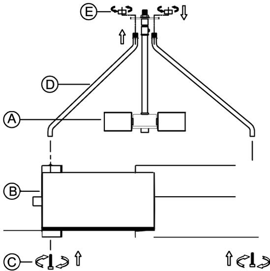
3. Attach round arm (D) to frame (B) use screw (C) to secure tightly; then attach other end of round arm (D) to the steel plate of fixture (A) use finial (E) to secure tightly.
