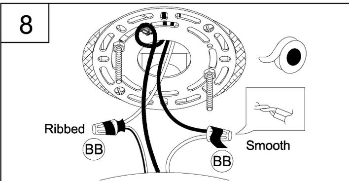
8. Strip 3/8" of insulation from the electrical wire ends. Using wire nuts (BB), connect RIBBED fixture wire to the WHITE supply wire from the outlet box; connect the SMOOTH fixture wire to the BLACK supply wire.
