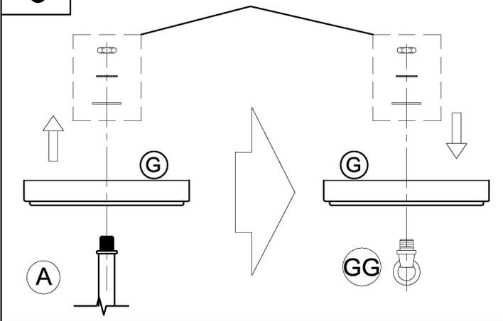
6. Remove existing canopy parts and canopy (G) from fixture(A).
