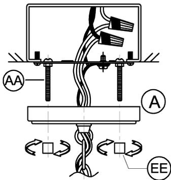
9. Secure the fixture (A) to screws (AA) use the two cylinder nuts (EE) to secure tightly.
