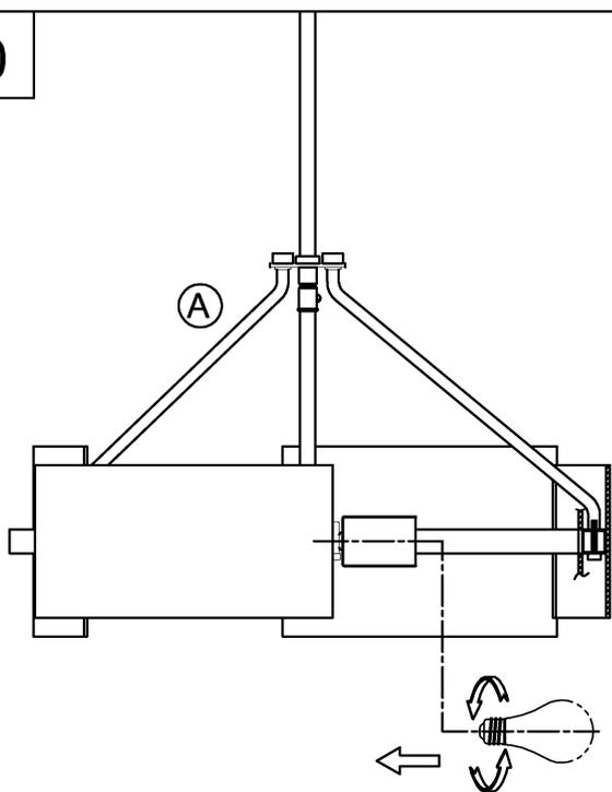
10. Screw lamp (not included) into fixture socket. Use 60-watt MAX incandescent medium base lamp, SBCFL or SBLED.
