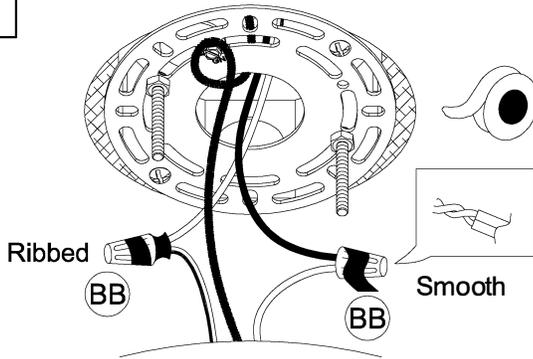
4. Strip 3/8" of insulation from the electrical wire ends. Using wire nuts (BB), connect RIBBED fixture wire to the WHITE supply wire from the outlet box; connect the SMOOTH fixture wire to the BLACK supply wire. Connect the fixture ground wire and supply ground wire using a wire nut or by fastening to the ground screw on the round mounting plate. Push all wire connections into the outlet box.
