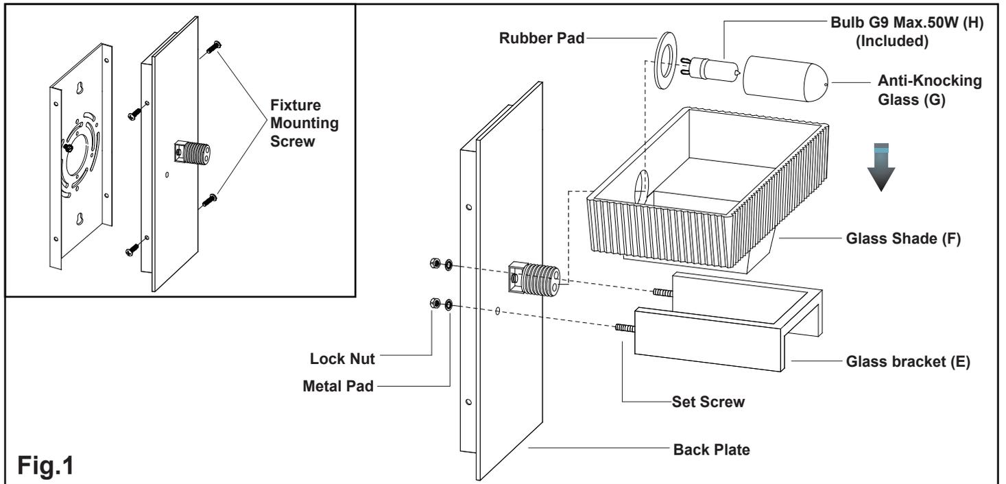
1. Unscrew four fixture mounting screws, and remove the mounting plate from the back plate.
