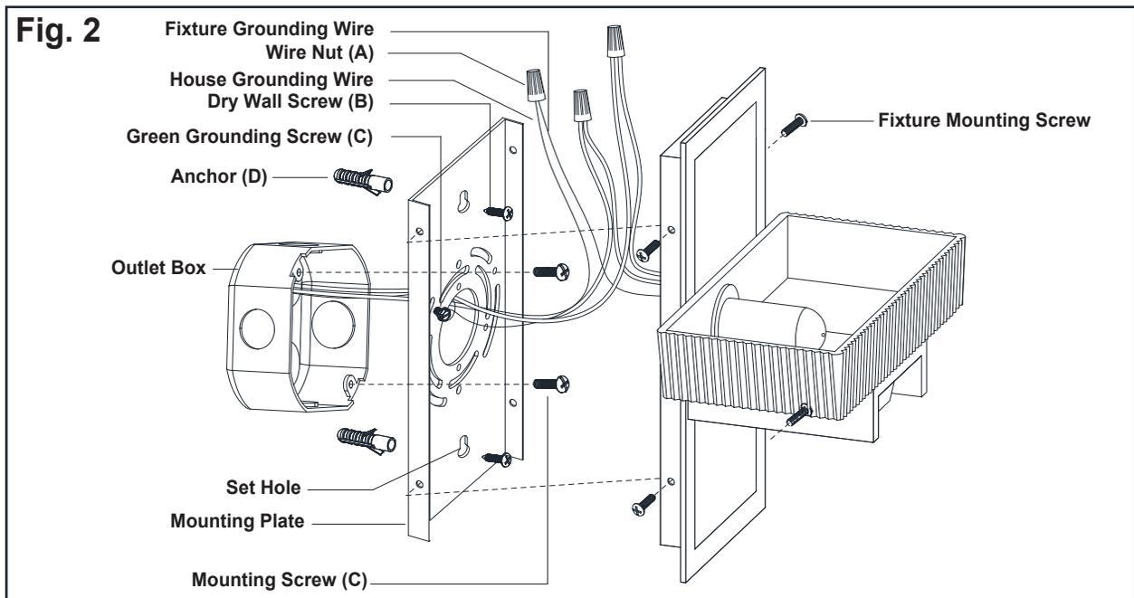
6. Attach the mounting plate to the wall.
